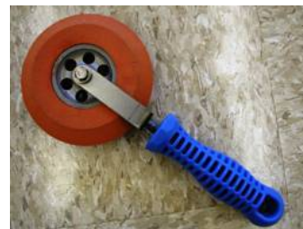
TSA-2 Tool for application in mortar lines
